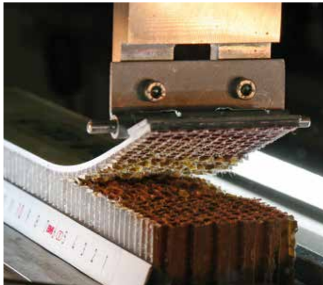
Experimental setup of a single cantilever beam test (SCB) for a sandwich sample with a honeycomb core
