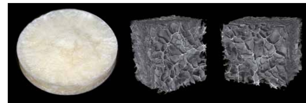
left: macroscopic image of a round elastin / gelatin sponge (semi-finished product for a wound dressing) with a diameter of 4 cm. Right next to it: (2 cubes) micrographs of this sponge can be seen, showing the porous structure of this sponge. The edge length of the cube is 5 mm.
