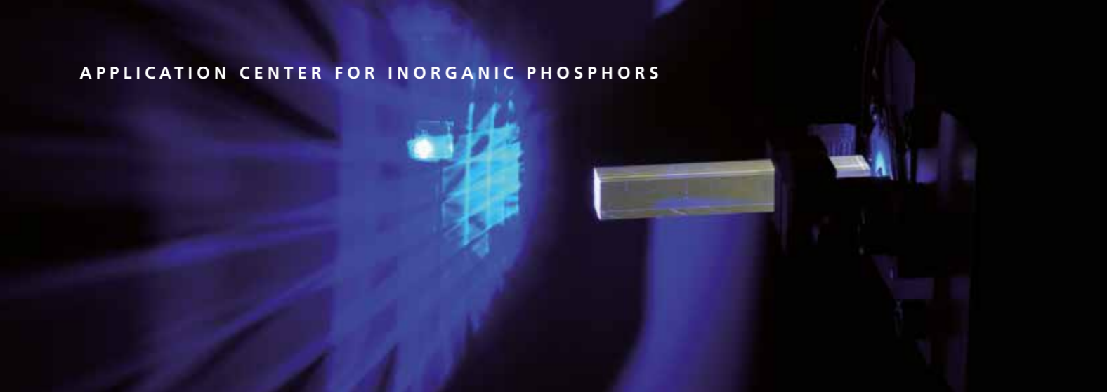
Dysprosium-doped glass rod glowing white under blue light excitation
