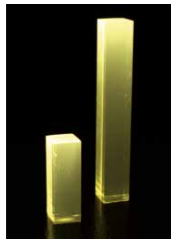
A glass rod made of dysprosium-doped borate.
