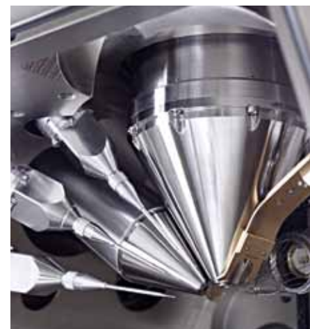
Devices producing focused ion beams are used to achieve the precise ablation of materials.
