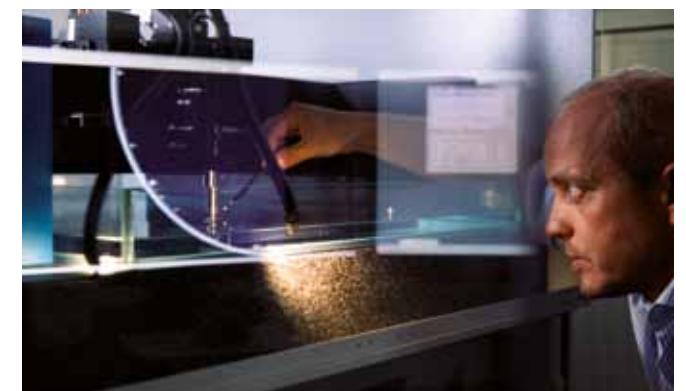
An acoustic microscope enables the tiniest cracks in materials to be detected without destroying samples.
