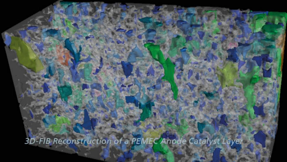
3D-FIB Reconstruction of a PEMEC Anode Catalyst Layer
