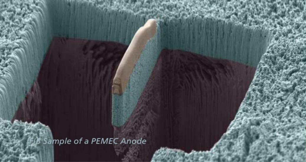
FIB Sample of a PEMEC Anode
