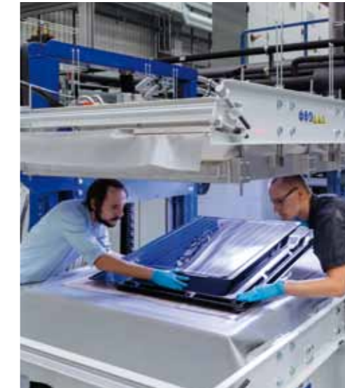
Fraunhofer CSP conducts lifecycle-relevant studies of module encapsulation stability in photovoltaic modules.
