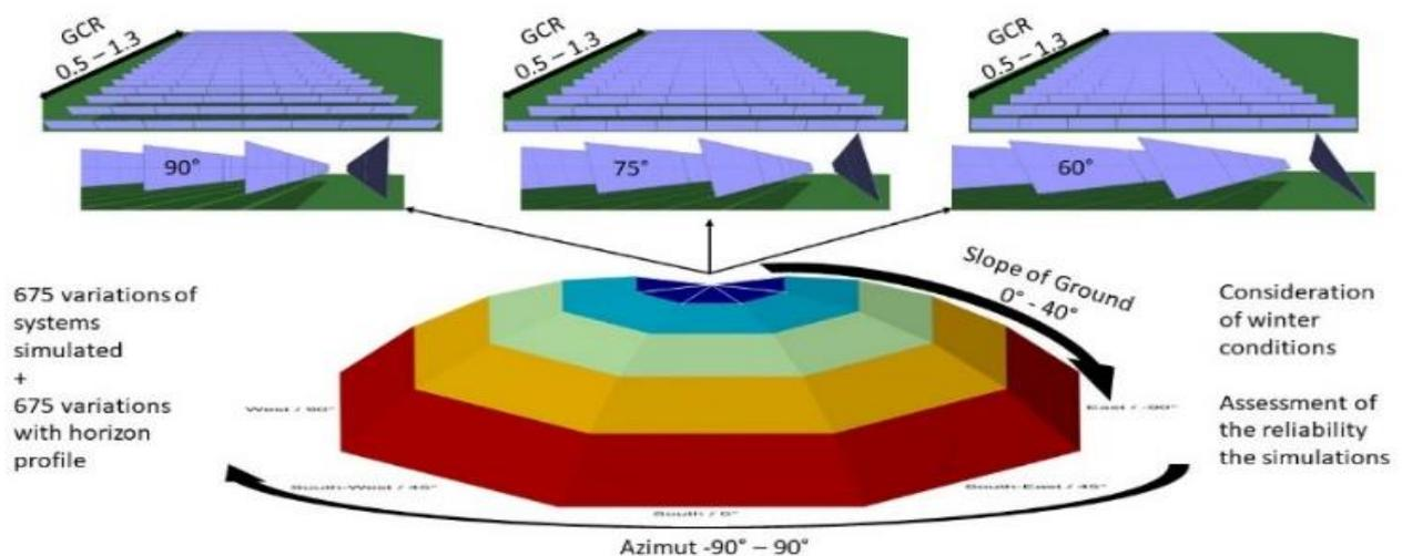
Figure 18: Systematic analysis of the System design.
