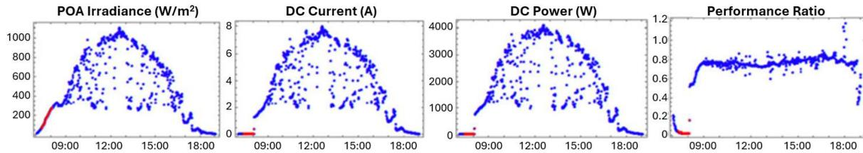
**Figure 36: Startup delay measured at floating PV in the Tengeh reservoir (Singapore) because of reduced insulation resistance. Source: SERIS**
