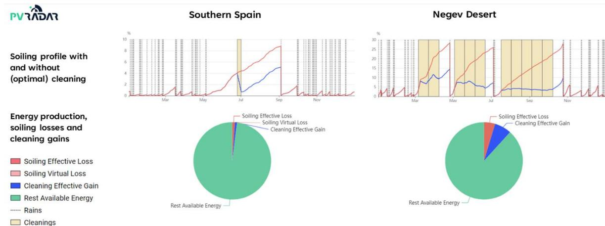
Figure 32: Direct comparison of optimal cleaning strategies for both sites, for one particular year. The exact cleaning dates (and number) changes depending on the expected rain patterns. “Virtual” gains and losses refer to energy that is lost due to inverter clipping. (Source: PVRADAR)
