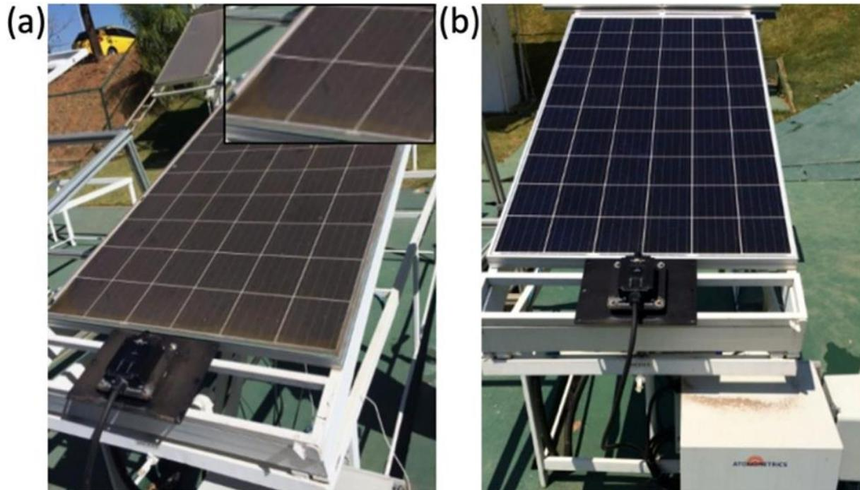
**Figure 39:** The monocrystalline soiling station installed in Belo Horizonte. In (a), the non-uniform soiling accumulated on the bottom frame at the end of the 85-day dry period. In (b), the clean module after a 20 mm rainfall [223].
