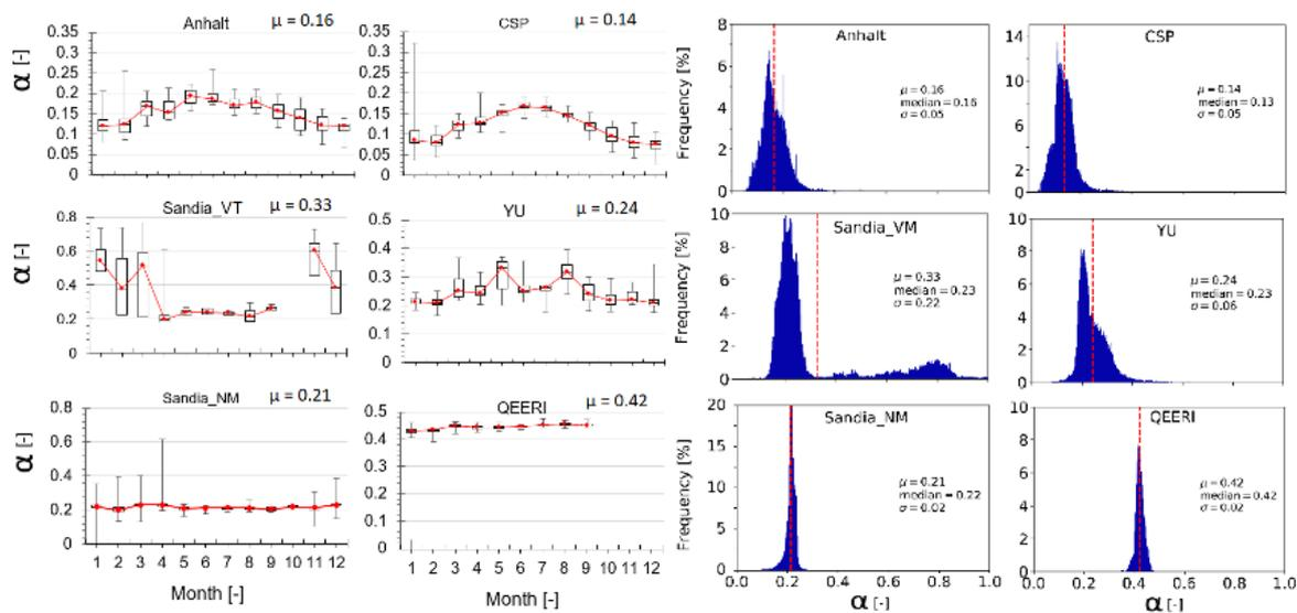
**Figure 7: PV CAMPER cross-climate albedo study. Results of one-year albedo data: (left) - Histogram of  $\alpha$  for each test site together with mean ( $\mu$ ), median and the standard deviation ( $\sigma$ ), (right) - Seasonal variation, monthly average of rear/front side ratio.**
