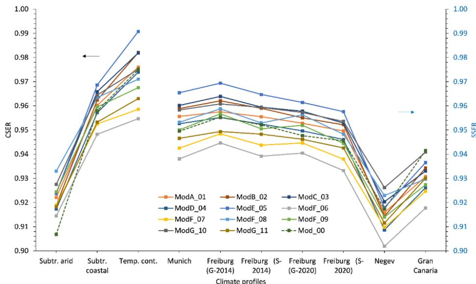
**Figure 5: CSER (left) and SSER (right) for 11 monocrystalline silicon PV modules from different manufacturers and a reference PV module (Mod\_00). Comparing Temperate continental-Munich/Freiburg, Subtropical arid-Negev, and Subtropical coastal-Gran Canaria. “G”: ground, “S”: satellite measurements [37].**
