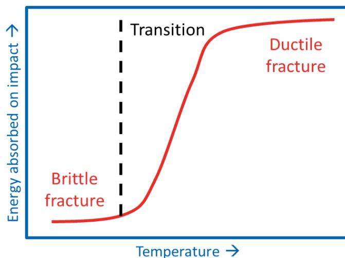
**Figure 14: Ductile-brittle transition temperature curve of polymers.**
