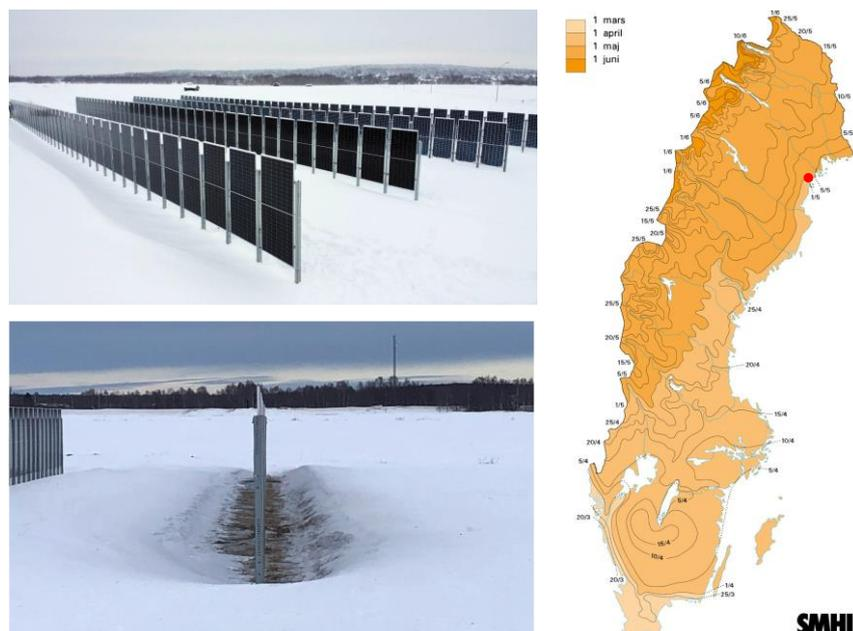
**Figure 21: Vertical bifacial 90 kWp PV system (Lilla Norrskenet) in Northern Sweden with pictures showing natural snow accumulation around the vertically mounted PV modules and the map of the last day of snow cover in Sweden from the SMHI (Swedish Meteorological and Hydrological Institute).**
