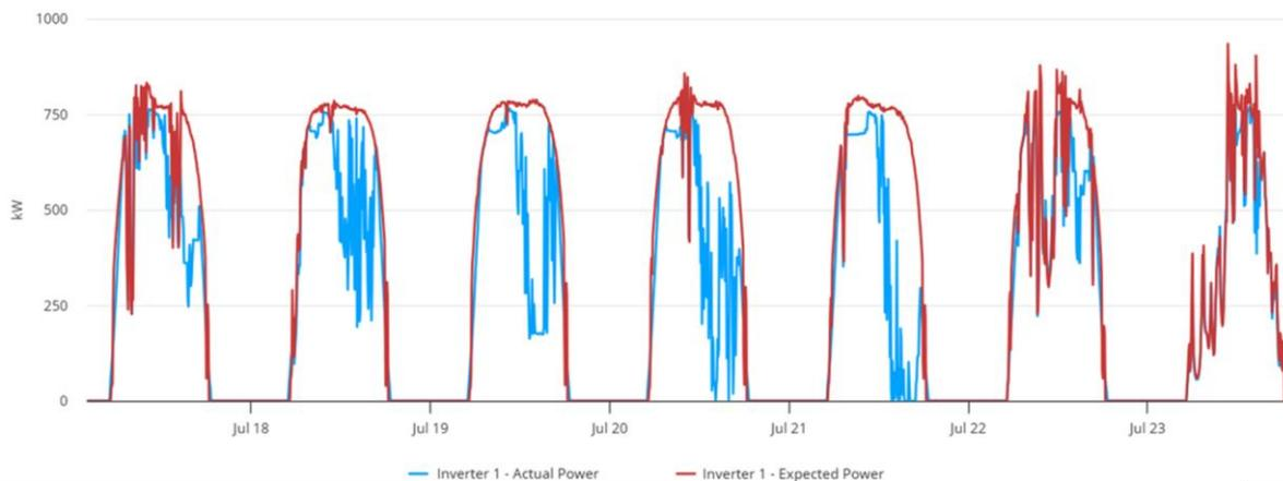
**Figure 27: Visualisation of measured and modelled active power of an inverter suffering from strong thermal derating (Source: Univers).**
