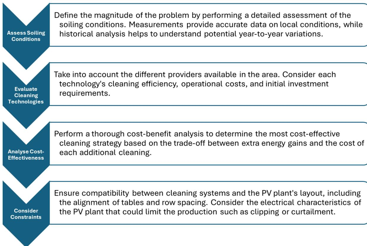
**Figure 28: Recommended Cleaning Optimisation Process (Source: PVRADAR).**
