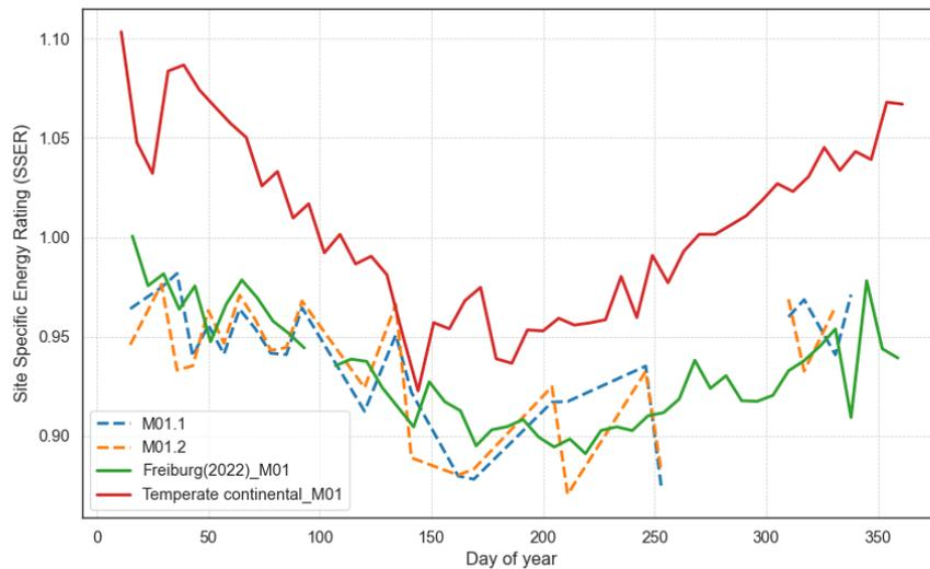
**Figure 4: Weekly *CSER* in Temperate continental (red),  $SSER_{MODEL}$  in Freiburg (green) and  $SSER_{REAL}$  (dashed lines) for a year of outdoor exposure between 2022-2023 with module manufacturer M01 (Modules M01.1 and M01.2) [36].**
