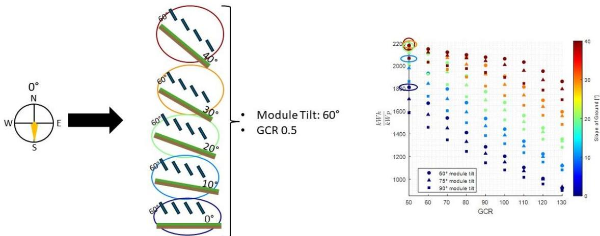
**Figure 19: Simulation results for annual specific yield at an azimuth of 0°.**
