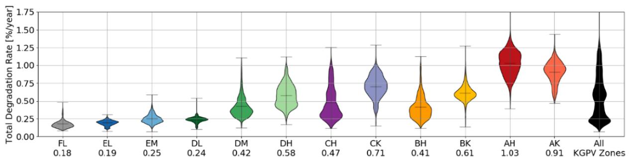
**Figure 6: Distribution of degradation rates in different KGPV climate zones (the average total degradation is indicated below in %/year). The width of each shape represents the density of degradation rates within each zone; wider sections indicate more frequent values. KGPV climate legend: A(tropical), B(desert), C(steppe), E(temperate), D(cold), F(polar), K(very high irradiance), H(high irradiance), M(medium irradiance), L(low irradiance) [41].**
