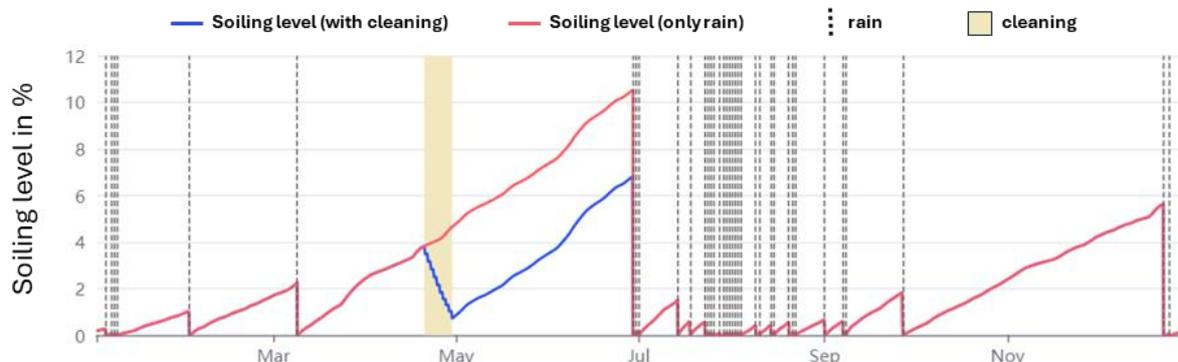
**Figure 29: Example of soiling levels with and without artificial cleaning, simulated with PVRADAR software. A longer dry period stretching from March to July is followed by two months of frequent rain. The blue line shows the soiling level if the systems is cleaned in April by the O&M team. The red line shows the soiling level if no artificial cleaning is performed (Source: PVRADAR).**
