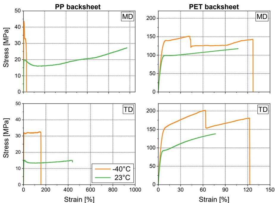
**Figure 15: Tensile test curves of PP and PET backsheets measured at  $-40^{\circ}\text{C}$  and  $23^{\circ}\text{C}$ , both in machine direction (MD) and transversal direction (TD) [83].**
