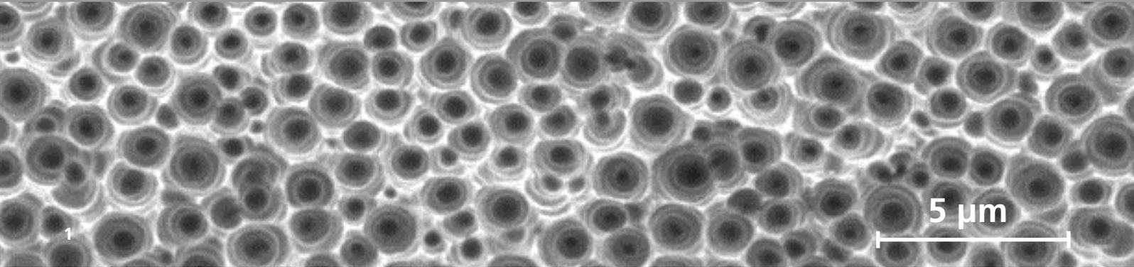
1 Top view of moth-eye structures for crystalline silicon solar cells. (SEM-image).
