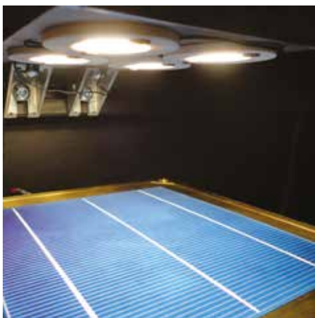
Figure 3. Test set-up of an LED-based light-induced (left) and electrical-induced (right) solar cell LID tester.
